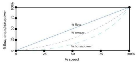
As a result of these relationships, we can see that a small reduction in the required airflow implies a large reduction in horsepower. In fact, running 2 motors at half speed requires less energy than running 1 motor at full speed.
